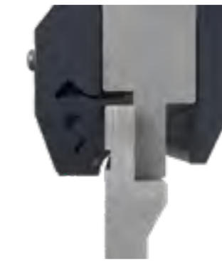
Insert the punch vertically
