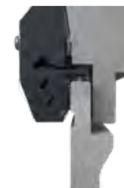
Rotate the punch by pushing the punch tip
