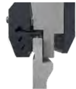
Rotate the punch by pushing the punch tip
