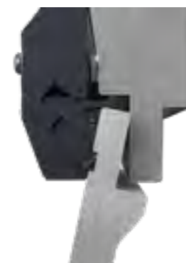
Pull the punch tip and when it's seated, pull it gently again until it reaches its working position
