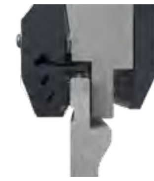
Pull the punch tip and when it's seated, pull it gently again until it reaches its working position
