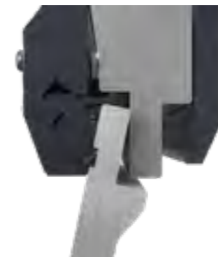
Pull the punch tip and when it's seated, pull it gently again until it reaches its working position
