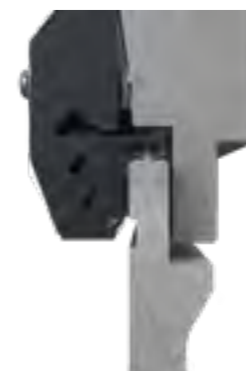
Pull the punch tip and when it's seated, pull it gently again until it reaches its working position
