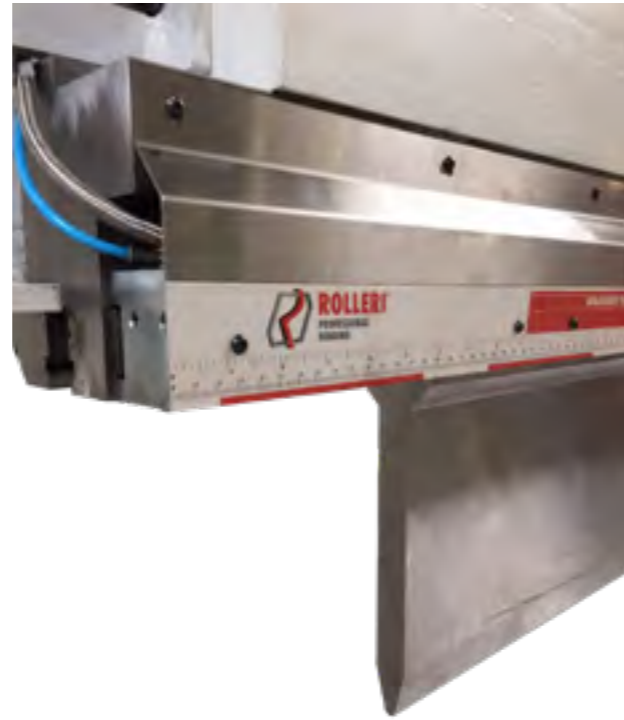
SPECIAL HYDRIBRID SYSTEM (Pneumatic and Hydraulic) 500 Tons/meter
