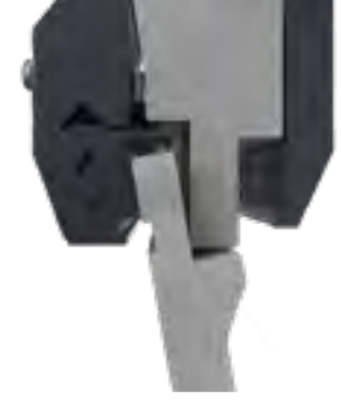
Rotate the punch by pushing the punch tip
