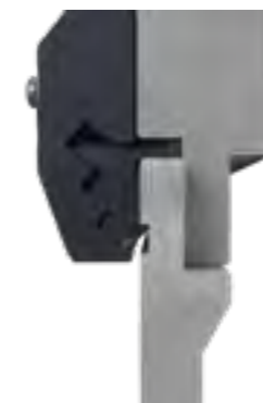
Insert the punch vertically
