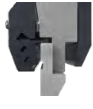
Push the punch against the intermediate by keeping it up
